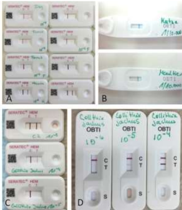
Figure 2. High Dose Hook Effect. (A) SERATEC HemDirect in different concentrations ( 10^{-1} , 20^{-1} , 50^{-1} and 10^{-2} ); (B) OBTI HEXAGON in different concentrations ( 10^{-1} , 20^{-1} , 50^{-1} , 10^{-2} and 10^{-3} ), a faint line appeared after 3h.
