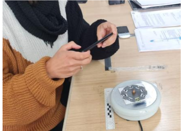
Figure 2. Rotary plate with a projectile being photographed with the round fixed scale.
